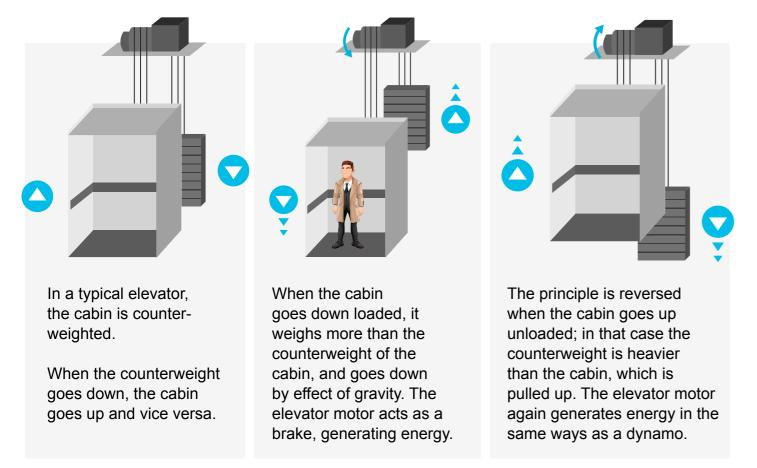
In electric traction elevators that include inverters, the generated energy is wasted as heat via the braking resistors. The ElevatorKERS stores the energy in Skeleton Technologies' supercapacitors until it is needed again to help power the elevator and decrease the use of energy from the grid.
