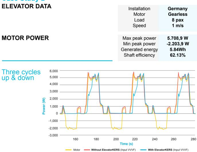
ElevatorKERS system to save and reuse the energy generated by the motor
