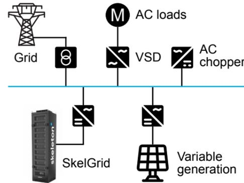
**Skelgrid connected to AC bus systems through DCAC Inverter**
